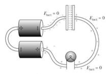
t = 100 s after starting (bulb is not glowing)
